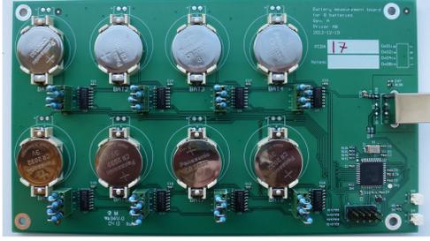
Fig. 3. Test card (Rev 2): The processor (bottom right) connects load resistors to each battery and records output voltage. Cost is  $<150\text{€}$ .
